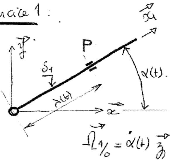
$$\vec{V}_{P/R} = \left[ \frac{dOP}{dt} \right]_R = \dot{\lambda}(t) \vec{x}_1 + \lambda(t) \dot{\alpha}(t) \vec{y}_1$$
