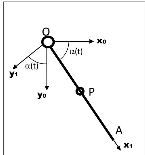
$$\Gamma \mathbf{P}/\mathbf{R}_0 = \lambda^{\circ\circ}(t) \mathbf{x}_1 + \lambda(t) \alpha^{\circ\circ}(t) \mathbf{y}_1 - \lambda(t) \alpha^{\circ 2}(t) \mathbf{x}_1 + 2 \lambda(t) \alpha^\circ(t) \mathbf{y}_1$$
